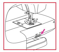
The drop feed lever can be seen on the base at the back side of the sewing machine.
