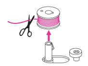
8. Cut the thread and then remove the bobbin.
