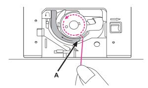
With a finger hold gently on top of the bobbin, please follow the arrow markings and draw the thread into the bobbin thread guide from (A) to (B).
