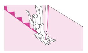
This foot has a groove on the underside which allows dense stitching to pass freely underneath.
