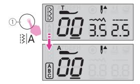
The LCD screen will be set at Regular Pattern Group. By pressing the pattern group switch button to select the stitch mode.
