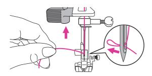
14. Hold the thread loosely and release the lever slowly. The hook turns and passes the thread through the needle eye forming a loop.
